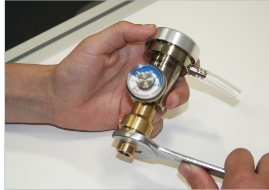
Fig. 18: Tighten adapter with wrench
