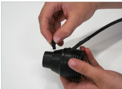
Fig. 07: Close opening for sample line
