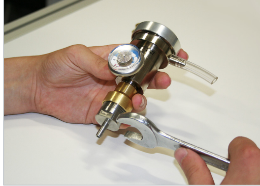
Fig. 22: Screw the tube adapter together with the gas-on-demand valve
