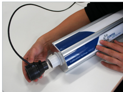
Fig. 08: Connect flow sensor with calibration pump
