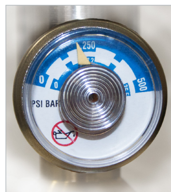
Fig. 20: Readout on the pressure valve displays 12 bar or 250 PSI an.
