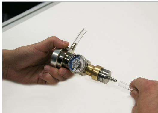
Fig. 23: Plug tube into tube adapter
