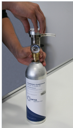
Fig. 19: Screw the gas-on-demand valve on to the CORTEX sample gas bottle
