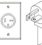
Type: Hospital Grade, NEMA 6-20R Contact, Arrangement, Isolated Ground Voltage Rating: 250 Volts, 20 AMPS Input Frequency: 60Hz (international 50Hz available) Color: Orange Dimensions: 2 5/8" L x 1 35/64" W Contact Material: Solid Brass Note: Ground is positioned at the top
