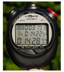
Top display shows cumulative time to last split. Middle display shows previous split lap time. Bottom display shows the cumulative running time
